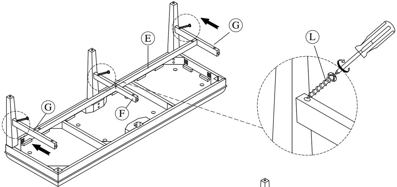
STEP 4 : Using the Allen key to tighten all bolts.
