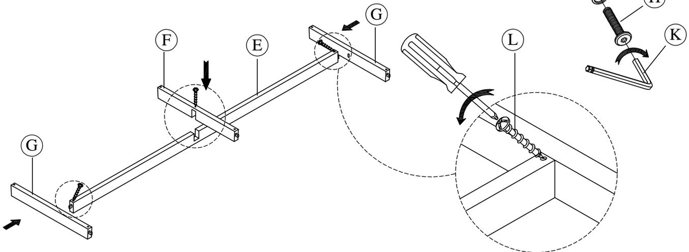
STEP 3: Do not fully tighten all Screws.
